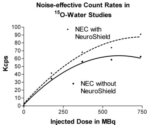
Fig. 5. NEC rates in bolus water studies with and without NeuroShield in place.
