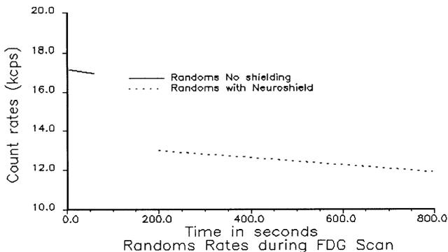
Fig. 6. Random count rate during the first minute of an FDG scan without NeuroShield, and for ten minutes with the NeuroShield in place.
