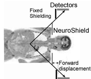
Fig. 1. Shielding geometry of the NeuroShield for the CTI ECAT HR+ fixed front collimators. The further forward the NeuroShield is with respect to detectors, the better the shielding. Without the NeuroShield in place the detectors are in the direct path of rays from the heart. (The fused PET-CT image was reproduced from the General Electric Medical Systems web-site.)
