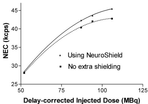
Fig. 7. NEC rates with and without the NeuroShield during FDG scans.
