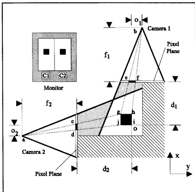
Fig. 3: Geometry used to calibrate the cameras. A block of known size is placed in the cameras' FOV. The resulting image is shown on the monitor. C1 and C2 correspond to images from camera 1 and 2 respectively. The hatched region is not displayed on the monitor (because of the video splitter) and is outside the FOV of the cameras. The dotted regions are seen by only one camera and thus are outside the FOV.
