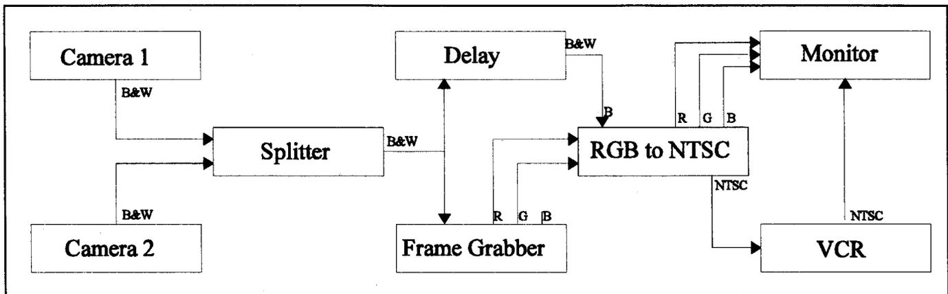
Fig. 2: Diagram of the video system. The connections are made using 75 ohm cables. R = red, G = green and B = blue.
