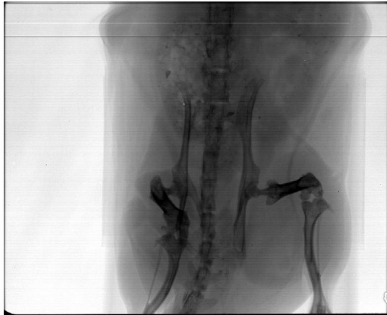
Figure 2.13. A raw exposure image. Note the detective columns and the non-uniformity wherein the image is brighter at the bottom than at the top.
