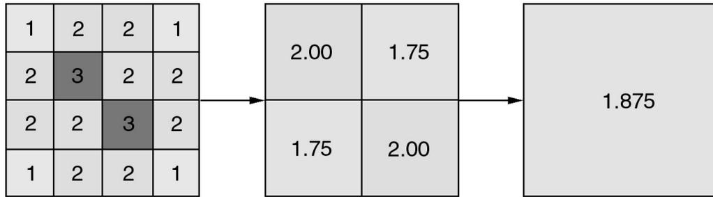
Figure A.2. Rebinning a phantom onto a coarser matrix by summing small voxels into larger ones. Each rebinning increased the length of a voxel side by a factor of 2.
