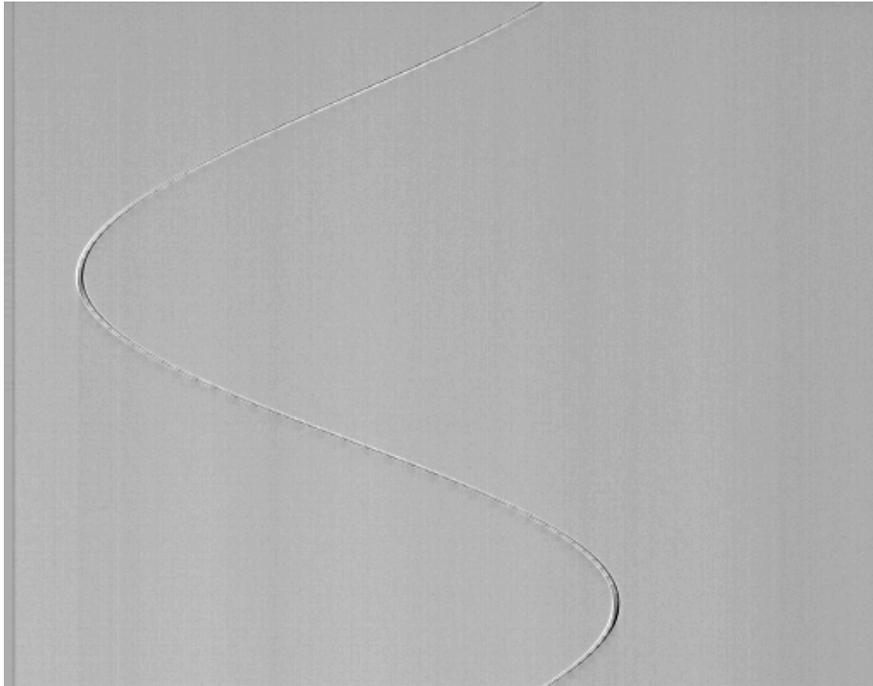
Figure 2.18. A subtraction of a simulated sinogram from a measured sinogram.
